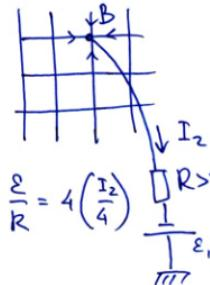
$$I_2 = \frac{\Sigma}{R + R_{AB}} = \frac{\Sigma}{R} = 4 \left( \frac{I_2}{4} \right)$$
