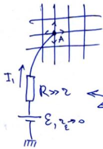
$$I_1 = \frac{\Sigma}{R + R_{AB}} \approx \frac{\Sigma}{R} = 4 \left( \frac{I_1}{4} \right)$$
