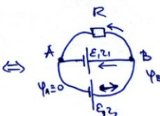
$$\left. \begin{array}{l} I_R = \frac{\Phi_B}{R} \\ I_1 = \frac{(\Phi_B - \Phi_A) - E_1}{Z_1} \\ I_2 = \frac{(\Phi_A - \Phi_B) + E_2}{Z_2} \\ I_2 = -\frac{\Phi_B + E_2}{Z_2} \end{array} \right\} \begin{array}{l} I_R = \frac{\Phi_B}{R} \\ I_1 = \frac{\Phi_B - E_1}{Z_1} \\ I_2 = -\frac{\Phi_B + E_2}{Z_2} \end{array}$$
